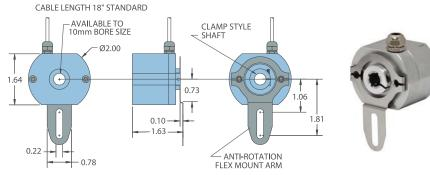
All dimensions are in inches with a tolerance of  $\pm 0.005$ " or  $\pm 0.01$ " unless otherwise specified.
